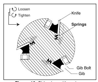
Figure 19. Side view with springs.
